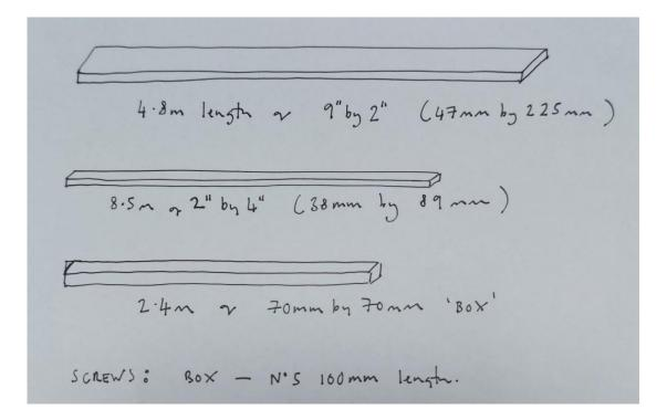
The work surface is made from one length of 4.8m 9by2. This is cut into 4 for the squarer workbench or into three for the longer rectangular version. (160cm x3 or 120cm x4)
