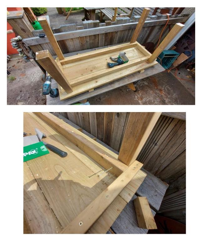
Add 5 screws into each leg – 2 on each side and one on diagonal
