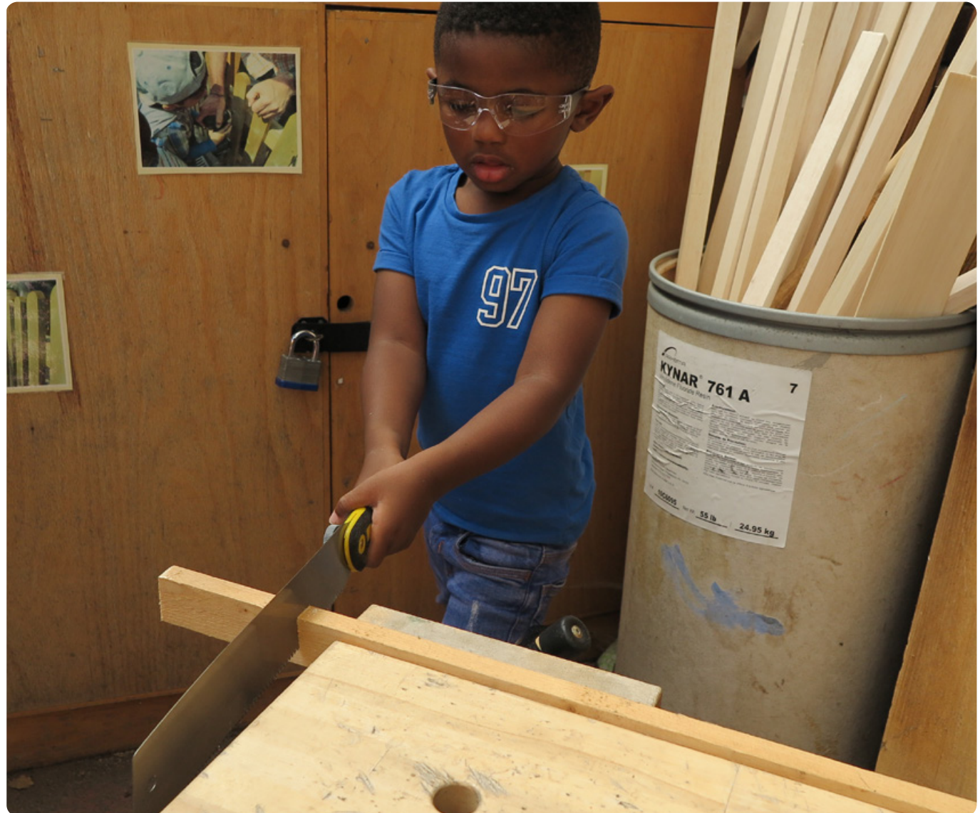
Fig. 33: Pull saws used with both hands are so much easier for young children to use and cut without snagging
